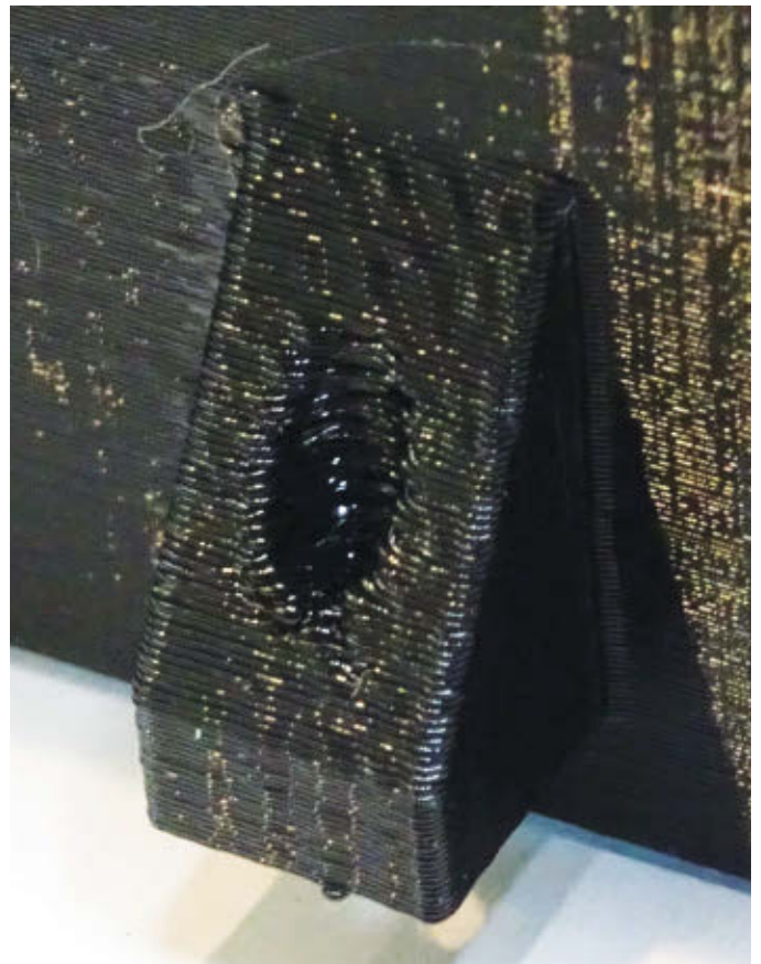
Figure 9 – Mounting tab on the bezel showing 4-40 thread printed in.
