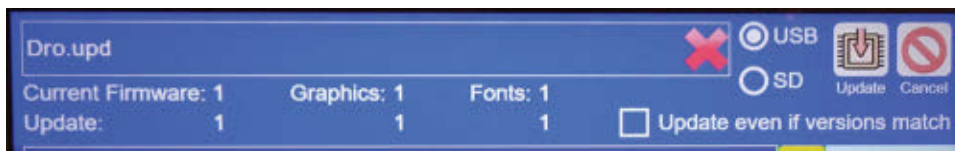
Figure 10 – The firmware update file has been opened and verified. You can compare the current DRO versions with those in the file.
