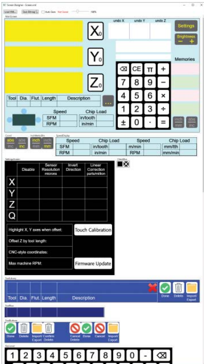
Figure 7 – Some of the graphic images for the DRO, which all get loaded into the 16 MB Flash memory.
