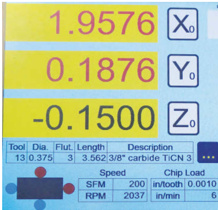
Figure 2 – Cutter radius offset is enabled for both the X and Y axes.
