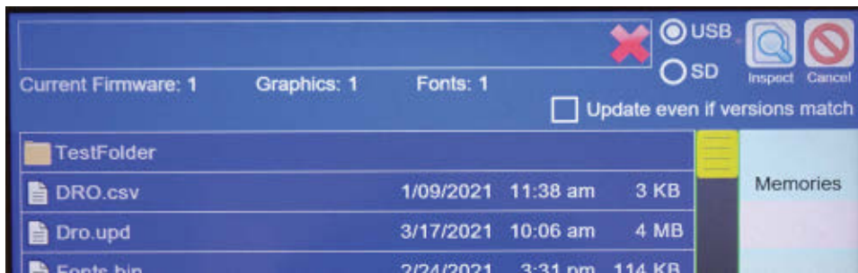
Figure 9 – Browsing for a firmware update file. It's the one with the ".upd" extension.
